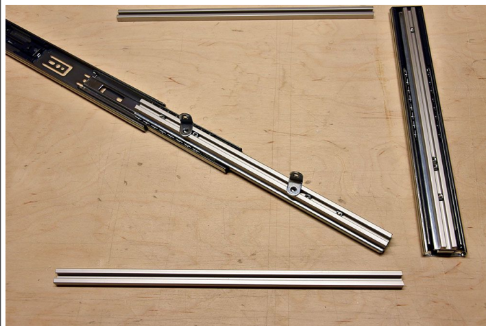
The four nuts for the drawer floor brackets are already in place in the rail
