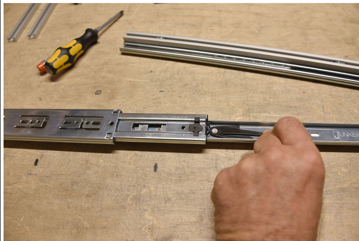
Unlock the telescopic profile drawer rail and pull out
