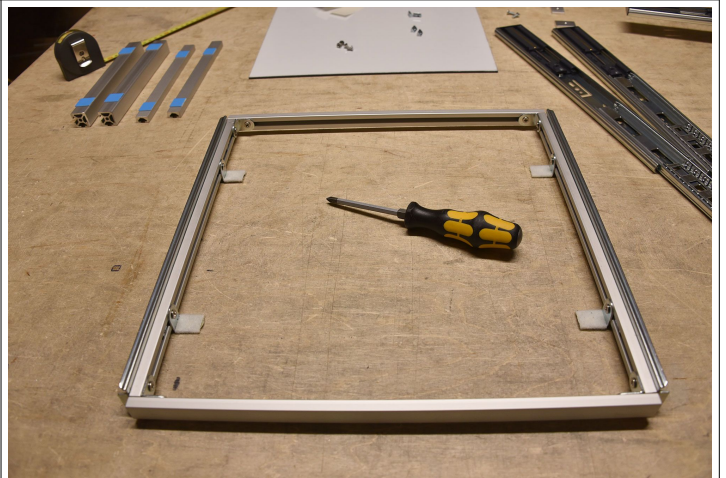
The finished drawer frame should look like this
