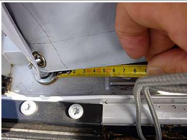
Affix the hook at the rear right. As per the latest version the loops will be hooked up - - - unlike shown in the figure with the eyelets - .
