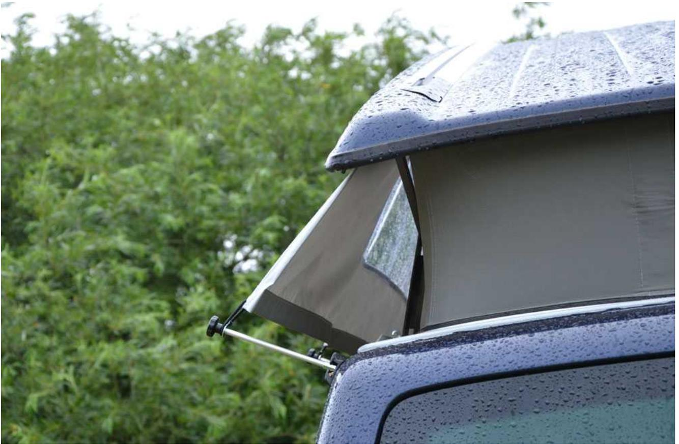
The stand-up installation will effect additional ventilation. These installations are not included with the items delivered.
