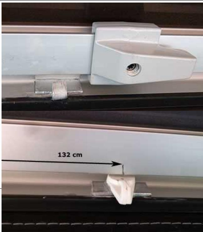
Adhere the aluminum hooks in the middle. Make sure to accurately observe the distance between the deadbolts.
