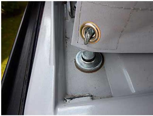
Affix the hook at the rear left. As per the latest version the loops will be hooked up - - - unlike shown in the figure with the eyelets - .
